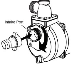
Slide one of the Hose Clamps over the end of the suction hose (a). Slide the Hose onto the Hose Coupler (b). Use a screwdriver (not included) to tighten the Hose Clamp until secure.
